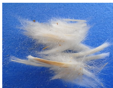
Fig.4 Recovered glass fiber from FRP using recycle solvent derived from the once liquefied FRP. H_2SO_4 (0.05 mmol/g) , 250°C, 240 min.
